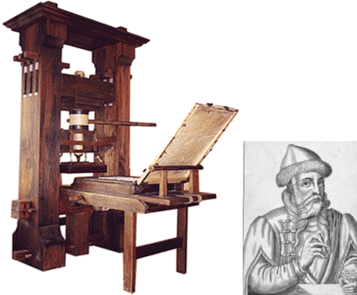
Figs. 16 & 17: The machine that changed it all (left), and the man who invented it. A replica of Gutenberg's original printing press, which made the mass production of books possible, and moved society from an oral to a literary way of thinking.
